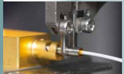
Active fiber (array) alignment
