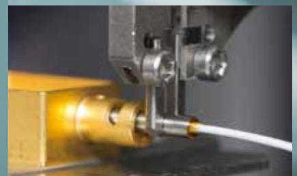
Active fiber (array) alignment
