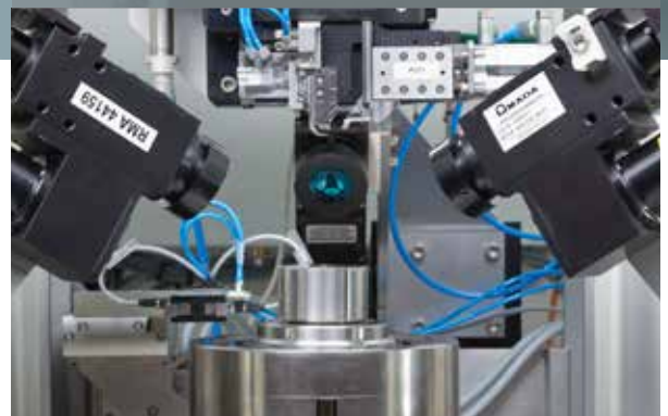
120° beam arrangement of laser weld heads
