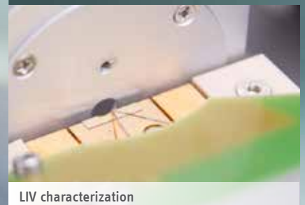
Dual fiber array alignment (active test)
